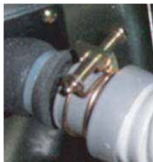
Clamp the Flexible Drain Hose Connection
