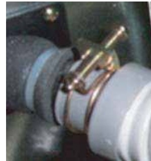
Clamp the Flexible Drain Hose Connection
