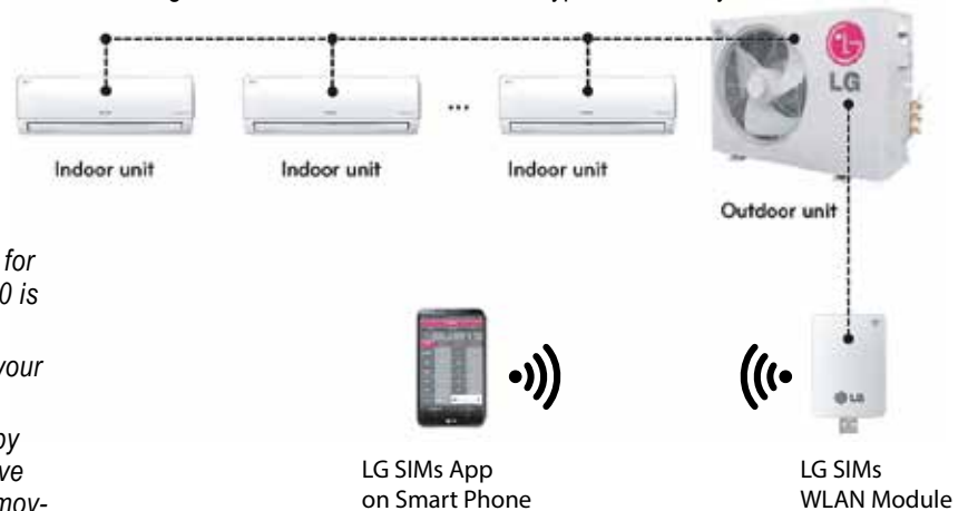
Figure 67: SIMs WLAN Module to a Typical Multi F System
